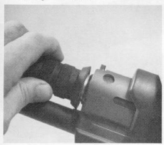
Remove the barrel assembly toward the front.
