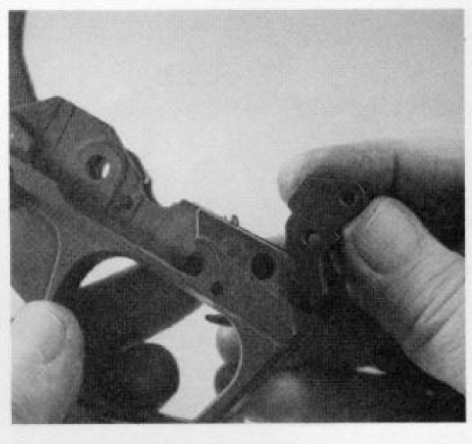
24. Remove the trigger upward.
