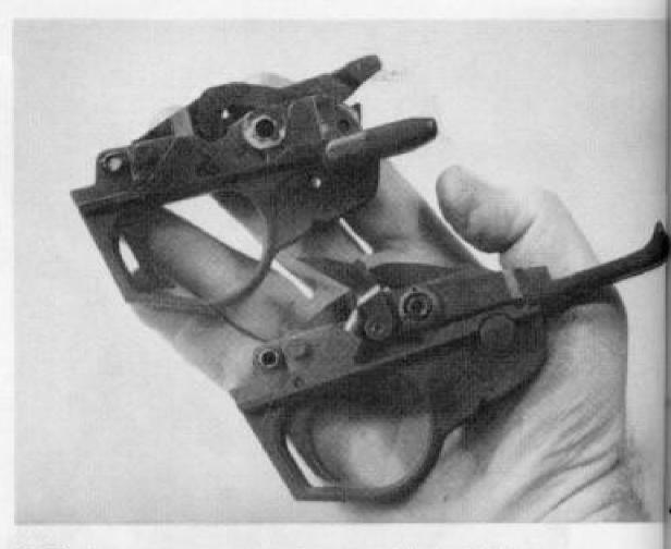
16. If you own a gun that has an original-style trigger group with two lever safety systems, like the one shown at top here, it should be sent to the importer and exchanged for the current version shown below it.
