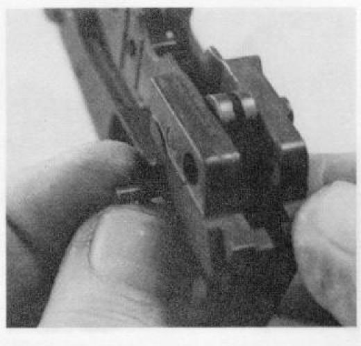
23. Push out the trigger cross pin.
