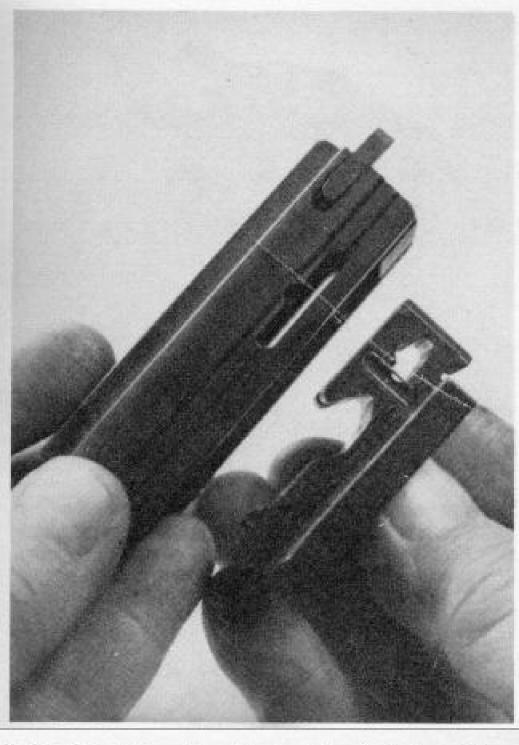
Detach the action slide piece from the bottom of the bolt. If necessary, the cocking handle retaining spring is easily removed from its recess in the slide piece.
