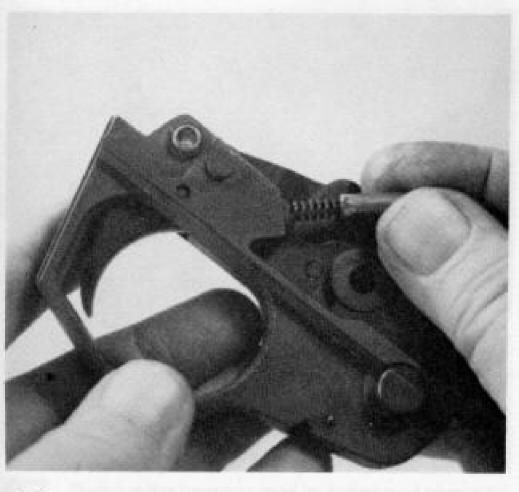
Remove the carrier plunger and springs. Note that there are two concentric springs, and take care that the smaller one isn't lost.
