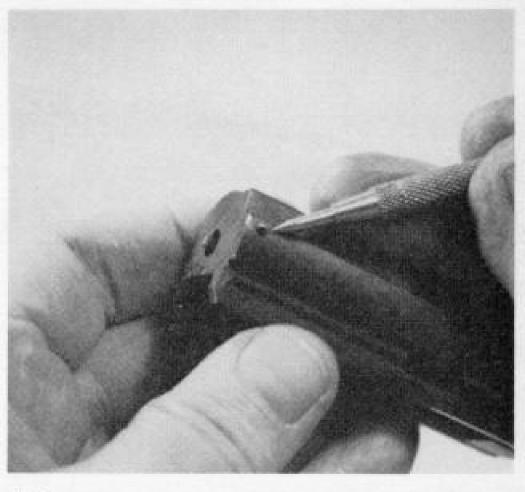
12. The firing pin and its return spring are retained by a cross pin that is drifted out toward the right. Removal of the firing pin will allow the locking block to be taken out upward. 13. The extractor and its plunger and spring are retained in the bolt by a vertical pin that is drifted out upward. Control the plunger and spring.
