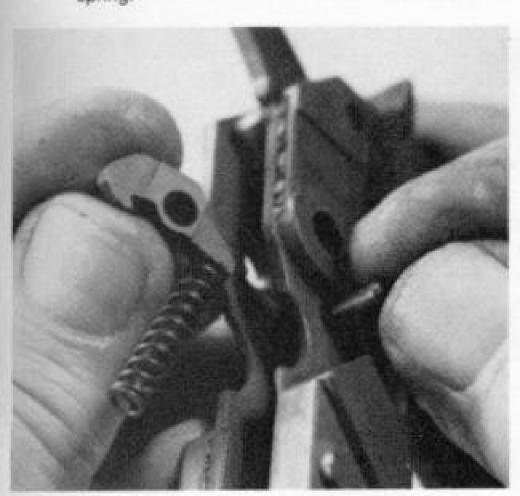
26. Restrain the hammer, and drift out the hammer pivot toward the left.
