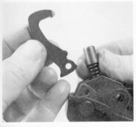
27. Remove the hammer, and its spring and plunger.
